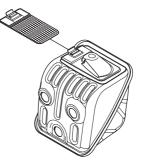
The muffler is designed to reduce the noise level and to direct the exhaust gases away from the operator. The exhaust gases are hot and can contain sparks, which may cause fire if directed against dry and combustible material.
